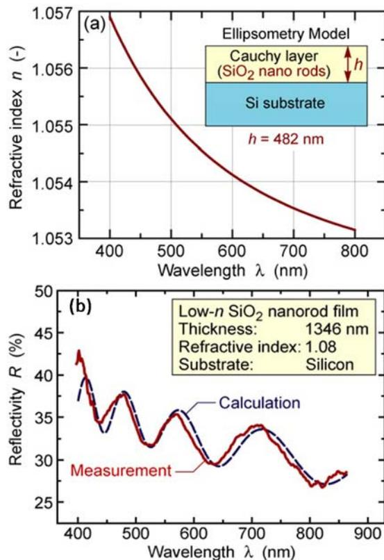
**Fig. 3.** (a) Refractive index dispersion curve of a low index SiO<sub>2</sub> nanorod thin film on silicon substrate as measured by ellipsometry, with (b) comparison of the measured and calculated reflectivity spectra.
