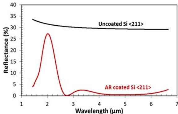
**Fig. 10.** Measured wavelength-dependent reflectance of multilayer AR-coated and uncoated Si<211> wafers. The multilayer AR coating on Si<211> shows average reflectance of 1.43% over the 3-5  $\mu\text{m}$  spectral band.
