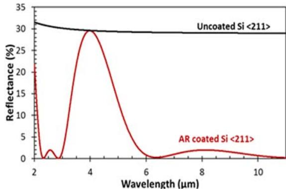
**Fig. 11.** Measured wavelength-dependent reflectance of two-layer AR-coated and uncoated Si<211> wafers. The two-layer AR coating on Si<211> shows average reflectance of 1.5% over the 8-10  $\mu\text{m}$  spectral band.
