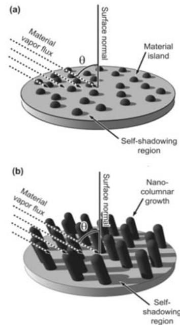
**Fig. 1.** Simplified schematic of the self-assembly process for synthesizing porous, nanostructured films, showing (a) the initial formation of material islands at random locations across the substrate, followed by (b) the formation of self-shadowed regions and nano-columnar growth when material vapor flux arrives at a non-normal deposition angle ( $\theta$ ) to the substrate.
