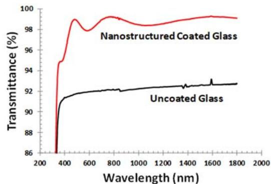
**Fig. 7.** Wavelength-dependent transmittance measurement of a step-graded, nanostructured SiO<sub>2</sub> AR coating on a glass substrate.
