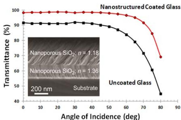
**Fig. 6.** Incident angle dependent broadband transmittance measurement through a glass slide coated on both sides with a step-graded, nanostructured SiO<sub>2</sub> AR structure. Also shown is the measured broadband transmittance of an uncoated glass slide, and a cross-sectional SEM image of a two-layer nanostructured coating.
