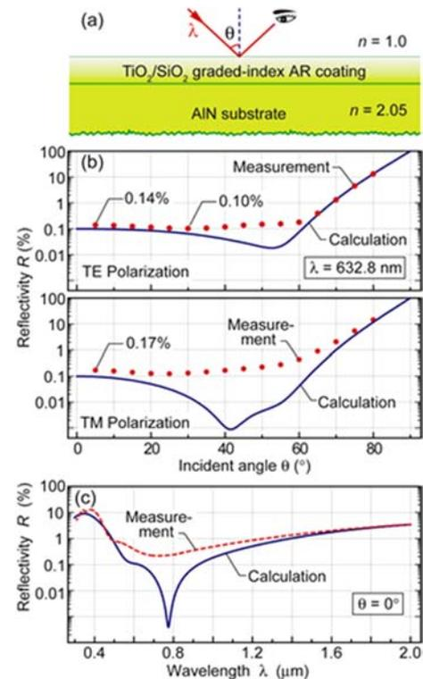
**Fig. 5.** Reflectivity of graded-index coating on AlN substrate summarized above in Fig. 4, including (a) schematic of the reflectivity measurement; (b) theoretical (solid line) and measured (dotted line) reflectivity of polarized light vs. incident angle; and (c) wavelength dependence of theoretical (solid line) and measured (dashed line) reflectivity at normal incidence. Further details can be found in Ref. [11].
