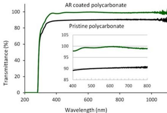
**Fig. 8.** Optical transmittance spectrum of a transparent polycarbonate sheet (5 mil thickness) before and after application of the large-area AR coating. The AR coating yields nearly 100% transmittance.
