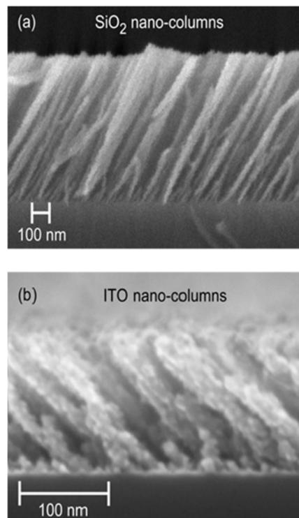
**Fig. 2.** Cross-sectional SEM images of nanostructured optical thin-films deposited by self-assembly process using (a) silicon dioxide, and (b) indium tin oxide materials.
