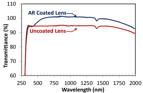
**Fig. 9.** Measured wavelength-dependent transmittance of a nanostructured SiO<sub>2</sub> coated lens compared to an uncoated lens. The AR coating yields nearly 100% transmittance. The ultrahigh transmittance was preserved for a wider spectrum of light.
