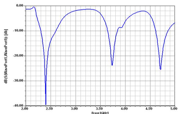
Fig. 2. C-type slot microstrip antenna return loss graph.
