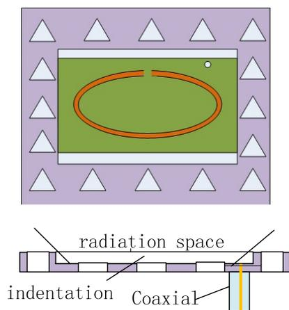
Fig. 4. PBG antenna top view and front view.
