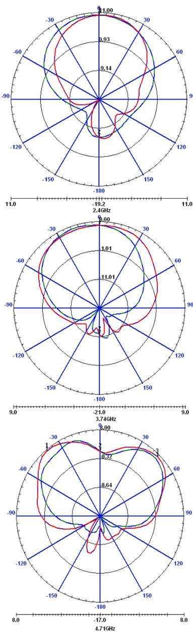
Fig. 3. C-type slot antenna radiation patterns microstrip.
