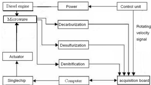
Fig. 1. Diesel engine exhausts gas detection system.
