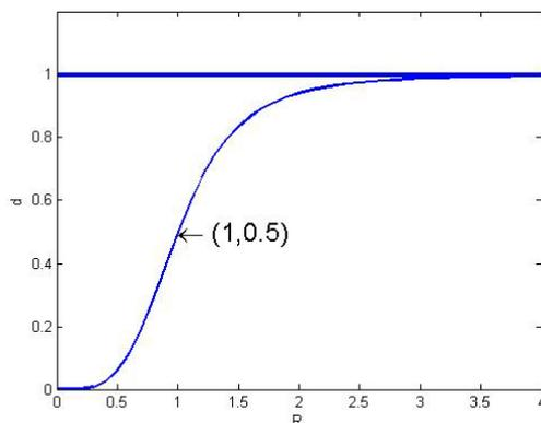
Fig. 3. The Butterworth filter function.
