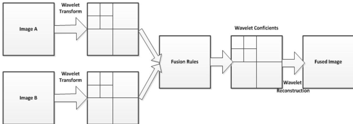
Fig. 1. Flow Chart of image fusion based on wavelet analysis.
