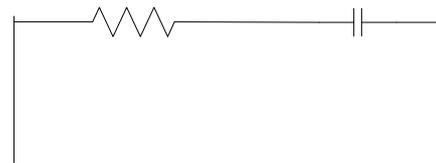
Fig. 2. Super capacitor equivalent RC model.
