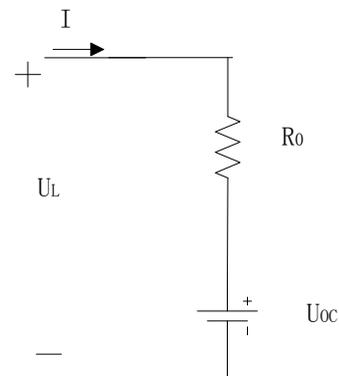
Fig. 3. Resistance equivalent circuit model.
