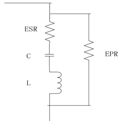
Fig. 1. Supercapacitor equivalent model.
