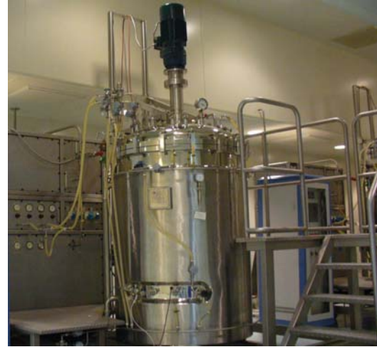
Fig. 5. WKT-30L fermentation experiment system.
