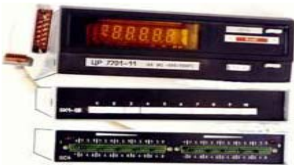
Fig. 2. Front view of universal digital multichannel measuring and signaling device CR7701.
