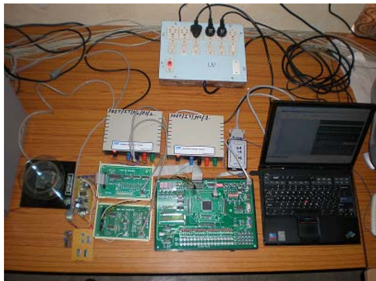
Fig. 10. Photograph of the experimental setup and working model of FPGA based DC motor speed control system.
