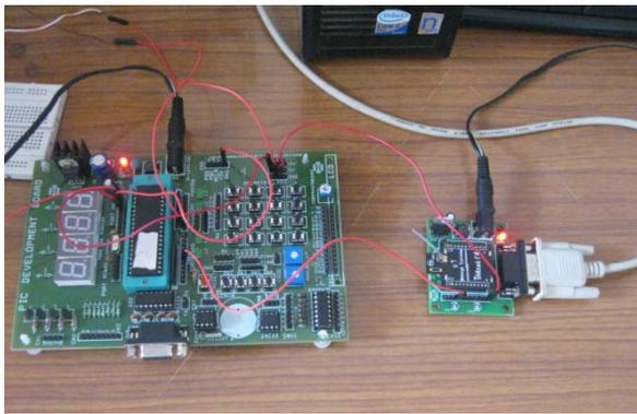
Fig. 8. Transceiver module with microcontroller board.
