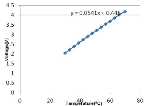
Fig. 7. Temperature vs. Output voltage.
