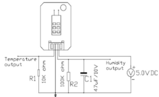
Fig. 4. Temperature and Humidity sensor HSM 20G.
