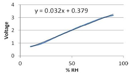
Fig. 6. Humidity vs. Output voltage.
