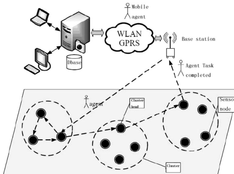
Fig. 1. Architecture of WSN and MA-based monitoring system.
