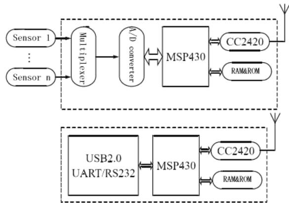
Fig. 2. Diagram of wireless sensor nodes and base station.
