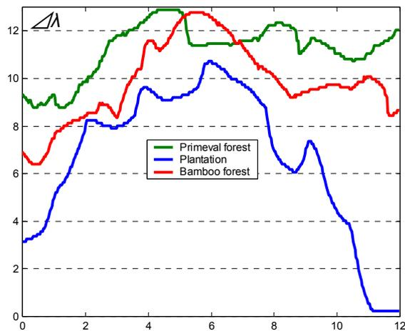
Fig. 4. 2.4 GHz electromagnetic wave attenuation curves within one year.
