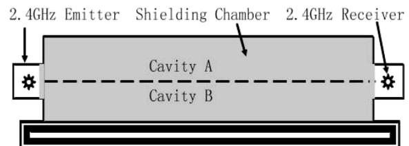
Fig. 3. GHz attenuation test bench for forest vegetation.
