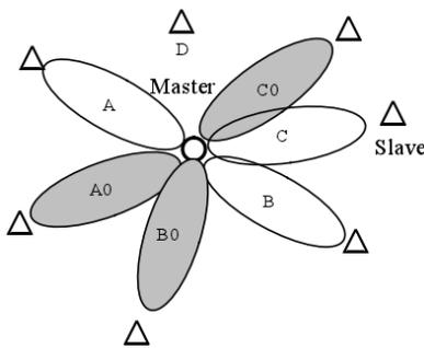
Fig. 5. Test schematic of Bluetooth Scatternet sensing channel.
