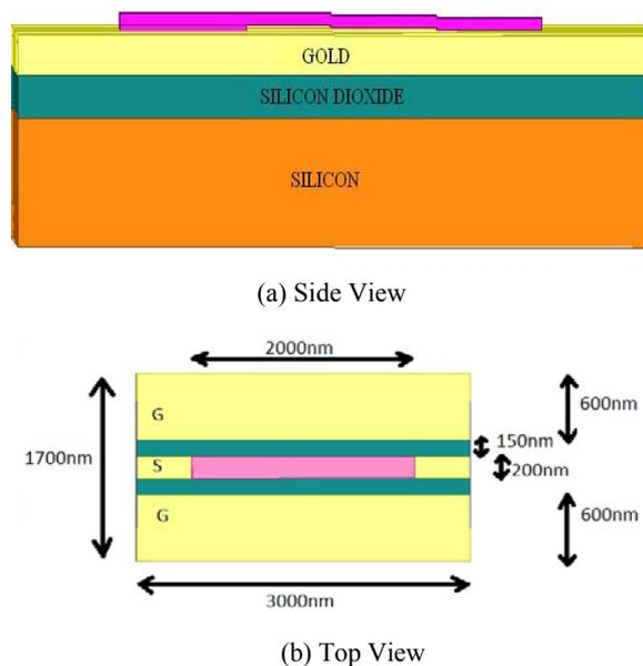
Fig. 1. Structural representation of the switch.
