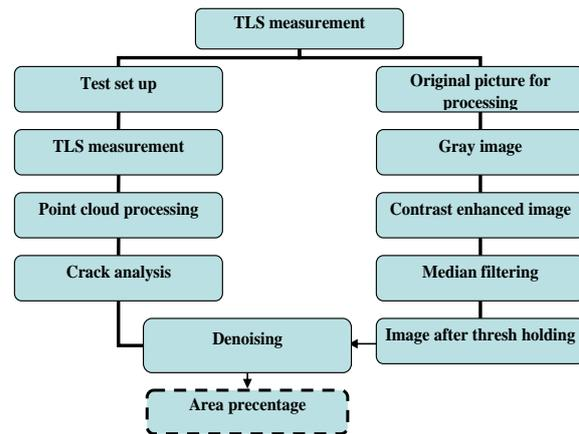
Fig. 1. The work-flow of crack analysis by MATLAB.
