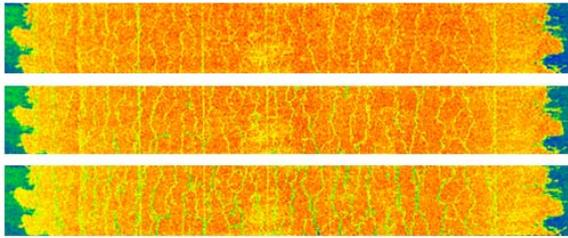
**Fig. 3.** The crack of concrete beam test by TLS.
