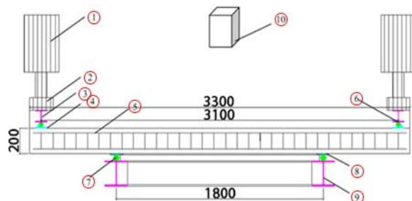
Fig. 2. Introduction of test setup [26]. Here: 1. Hydraulic jack; 2. Force sensors; 3. HEB 200 I-steel; 4. Steel plate of 5 mm; 5. Test specimen; 6. Steel tube (Diameter: 5 mm); 7. Steel tube (Diameter: 5 mm); 8. Steel plate of 5 mm; 9. I-steel frame (HEB 200); 10. Laser scanner.
