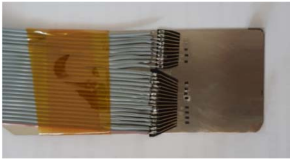
Fig. 4. Piezoresistor elements attached to a cantilever beam using different adhesives.
