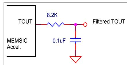
Figure 8: Temperature Output Noise Reduction
