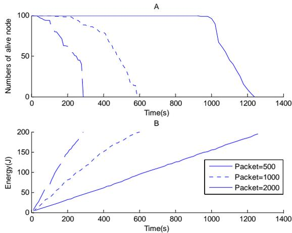
Fig. 9. The impact of different packet sizes on EEACH.
