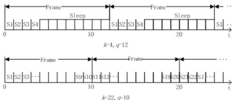
Fig. 5. The time slice planning of the minimal and maximal clusters.
