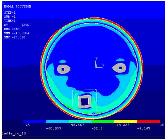
Fig. 3. The ladle after optimization thermal stress distribution cloud.
