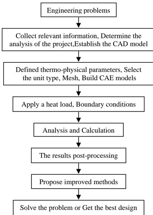
Fig. 1. ANSYS thermal analysis flowchart
