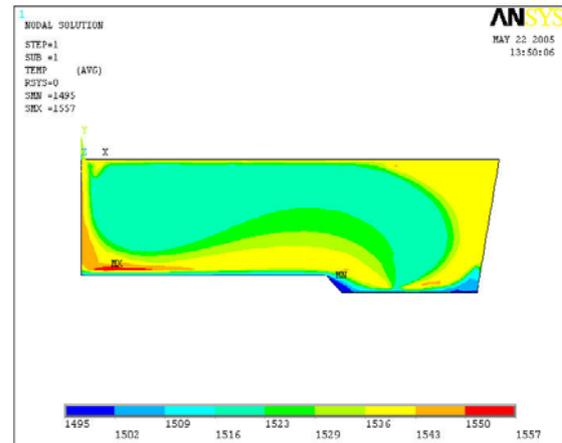
Fig. 4. The temperature isoline of molten steel in the no flow control device tundish.
