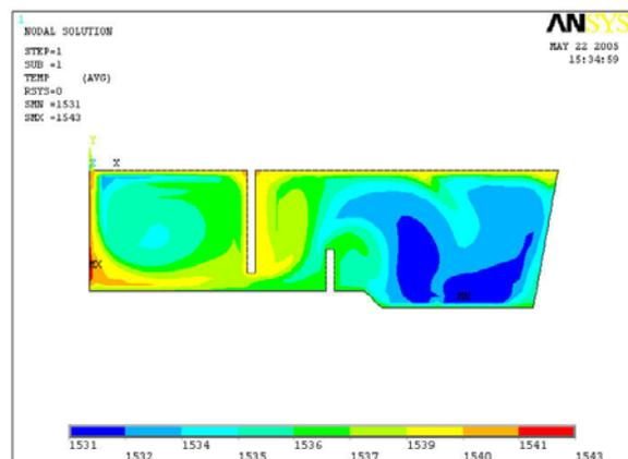
Fig. 5. The temperature isoline of molten steel in the tundish after setting the weir dam.
