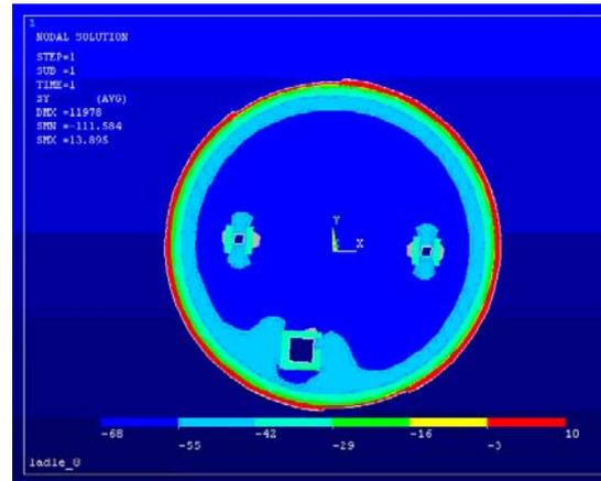
Fig. 2. The original ladle thermal stress distribution cloud.
