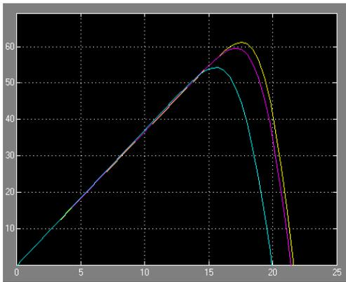
Fig. 4. Photovoltaic array P-V curve based on the change of temperature.
