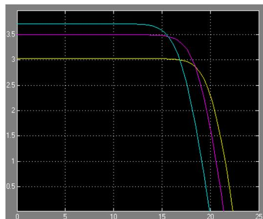
**Fig. 3.** Photovoltaic array I-V curve based on the change of temperature.
