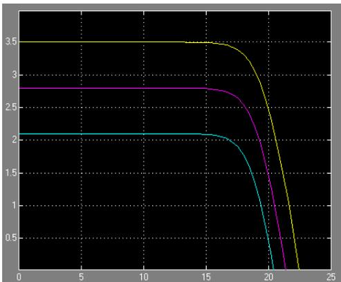
Fig. 5. Photovoltaic array I-V curve based on the change of sunlight intensity.
