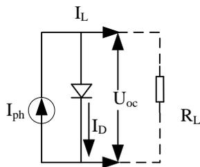
Fig. 1. Ideal equivalent circuit of the photovoltaic cell.
