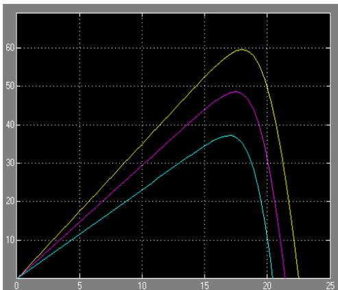
Fig. 6. Photovoltaic array P-V curve based on the change of sunlight intensity.
