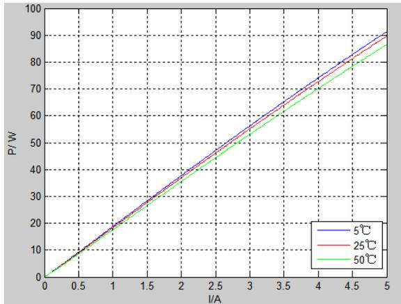
Fig. 7. Relationship of the maximum power point and the output current.
