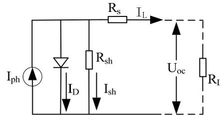
Fig. 2. Actual equivalent circuit of the photovoltaic cell.
