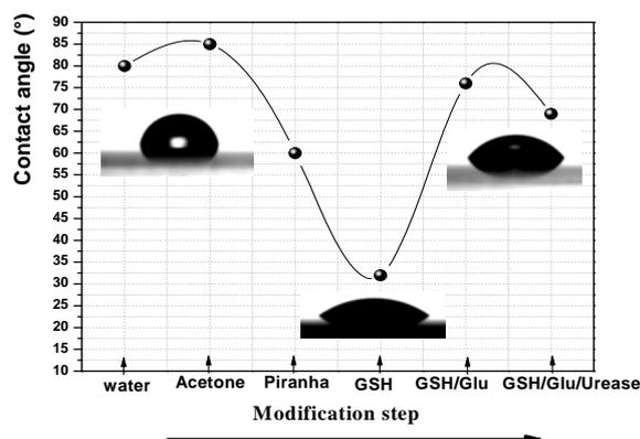
Fig. 6. Static contact angle variation during the building of the SAM system on the gold electrode surface.
