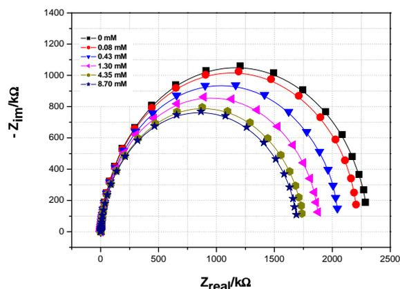
**Fig. 3.** Electrochemical impedance spectra of the Glutaraldehyde-Glutathione modified gold electrode in presence of different urea concentrations. 20 mM phosphate buffer containing 0.1 M of NaCl and pH=7.4, applied potential -0.3 V.
