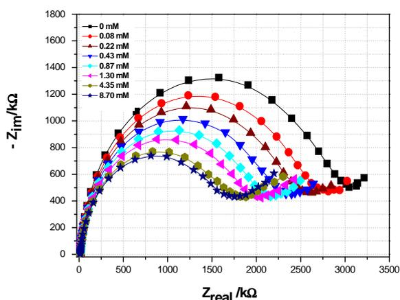
**Fig. 2.** Electrochemical impedance spectra of the Glutathione modified gold electrode in the presence of different urea concentrations. 20 mM phosphate buffer containing 0.1 M of NaCl and pH=7.4, applied potential -0.3 V.
