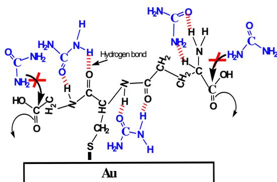
**Fig. 4.** A conceptual scheme of the Glutathione-Urea interaction via hydrogen bonds.
