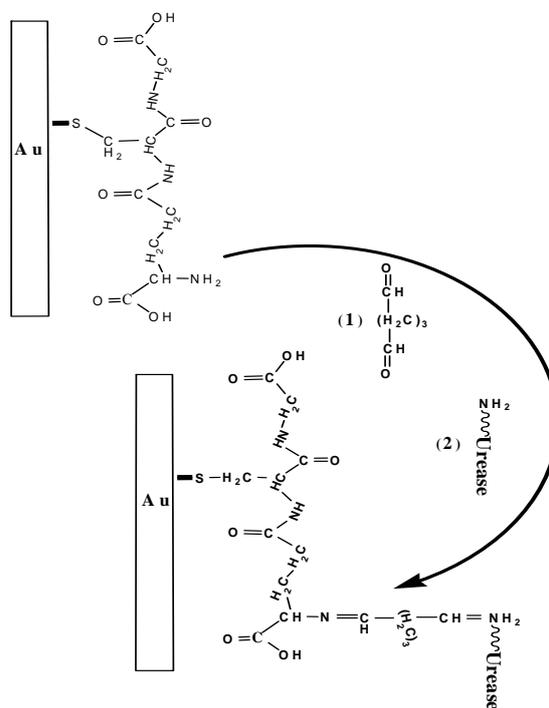
**Fig. 1.** Schematic representation of the immobilization of urease on gold electrode using a SAM of Glutathione via Glutaraldehyde as coupling agent.
