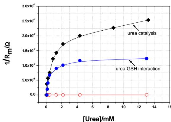
Fig. 8. Calibration plots of the membrane resistance variation as a function of the urea addition. (○) bare, (●) Glutathione/Au and (◆) urease/glutaraldehyde/Glutathione/Au electrodes. 20 mM phosphate buffer containing 0.1 M of NaCl and pH=7.4.
