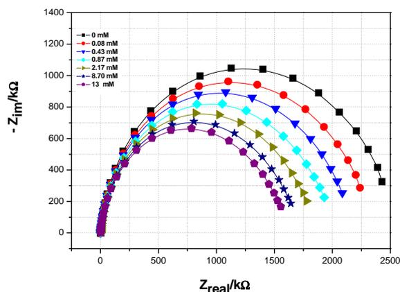
Fig. 7. Electrochemical impedance spectra of the Urease-Glutaraldehyde-Glutathione modified gold electrode in presence of different urea concentrations. 20 mM phosphate buffer containing 0.1 M of NaCl and pH=7.4, applied potential -0.3 V.
