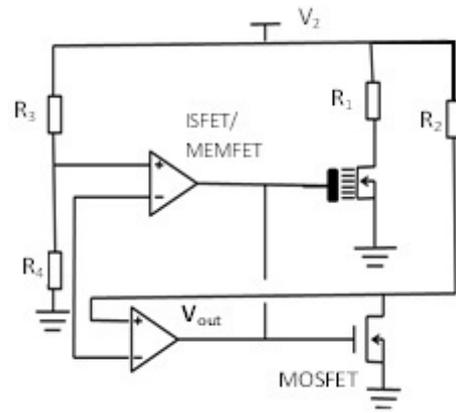
Fig. 6. Sensing circuit 1 based on a pair of ISFET/MEMFET and ReFET.
