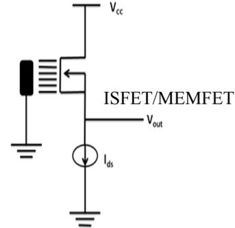
**Fig. 3.** Individual sensing circuit.
