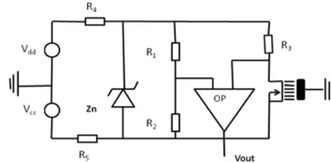
Fig. 10. Zener-based bridge-type sensing circuit.
