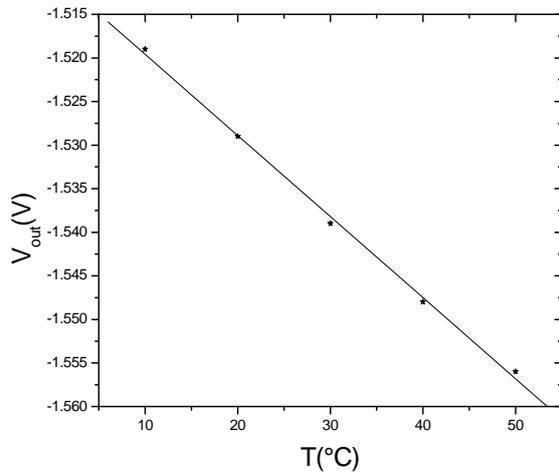
Fig. 5. Variation of  $V_{out}$  versus the temperature variation.
