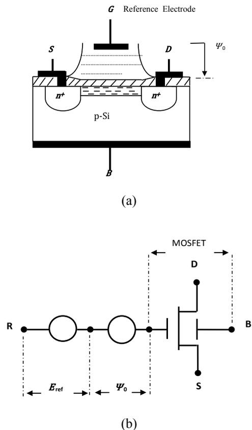
**Fig. 1.** (a) n-channel ISFET/MEMFET structure (b) Equivalent circuit of the ISFET/MEMFET.
