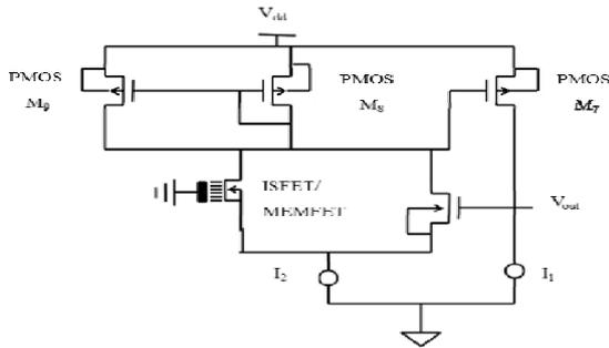
Fig. 8. Sensing circuit 2 based on a pair of ISFET/MEMFET and ReFET.
