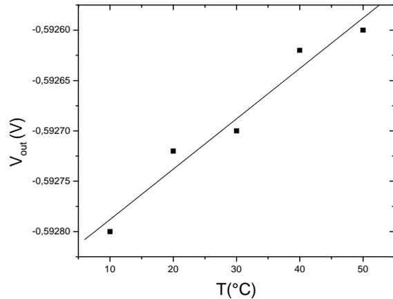
Fig. 14. Temperature's variation of the extracted signal  $V_{out}$ .
