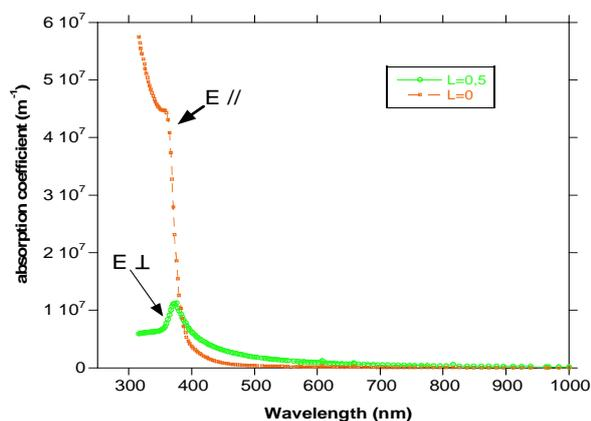
**Fig. 4.** EMT calculated absorption spectra of ordered SiNWs for longitudinal or transverse E polarizations. SiNWs fill factor = 0.8, in vacuum.
