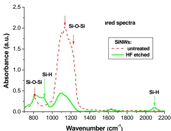
**Fig. 1.** Infrared spectra of as-produced and HF treated SiNWs showing the weakening of the Si-O-Si vibration modes and appearance of Si-H<sub>x</sub> modes upon SiO<sub>2</sub> sheath removal.
