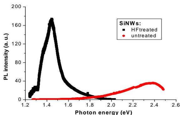
**Fig. 2.** PL spectra showing the disappearance of the peak at 2.38 eV attributed to SiO<sub>2</sub> centers and appearance of the silicon photoluminescence at 1.44 eV upon SiNW HF etching.
