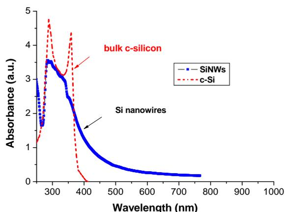
**Fig. 3.** Experimental UV-visible and EMT calculated SiNW absorption spectra.
