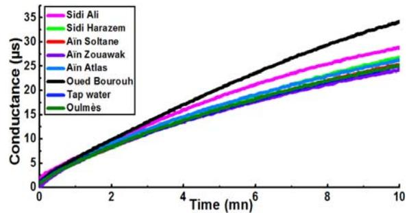
Fig. 3. Electrical conductance of TGS 842 sensor towards exposures to the studied waters.
