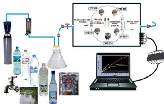
Fig. 1. Schematic representation of the experimental set-up of the electronic nose used in water measurements.
