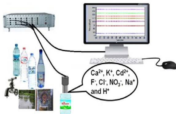
Fig. 2. Scheme of the potentiometric electronic tongue set-up.
