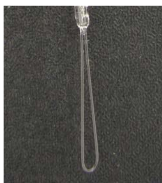
Fig. 3 (b). A photo of a sensing element with an arc diameter of 2 mm (a fiber diameter of 0.35 mm).
