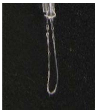
Fig. 3 (a). A photo of a sensing element with an arc diameter of 2 mm (a fiber diameter of 0.2 mm).
