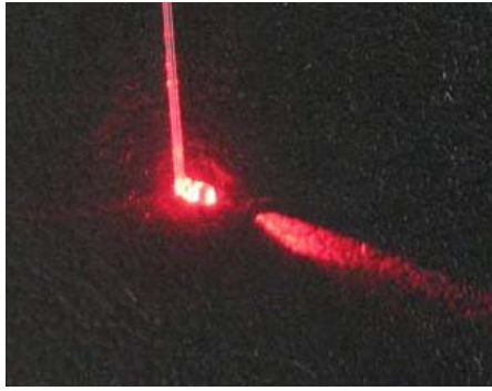
Fig. 3(d). A photo of a sensing element with an arc diameter of 0.3 mm (a fiber diameter of 0.35 mm).
