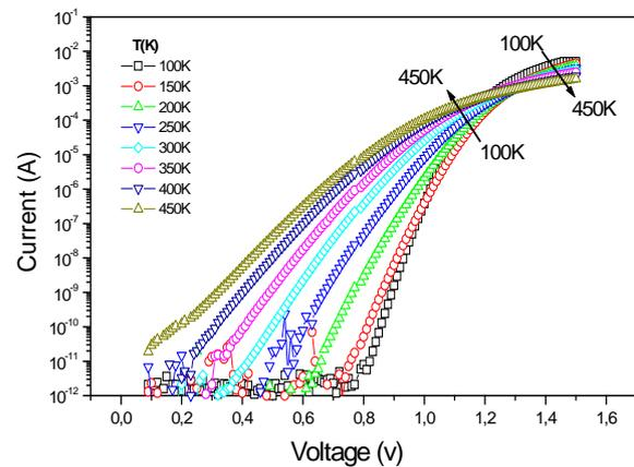
Fig. 2. Forward and reverse bias semilogarithmic I-V characteristics of a (Mo/Au)-AlGaN/GaN HEMTs at various temperatures.
