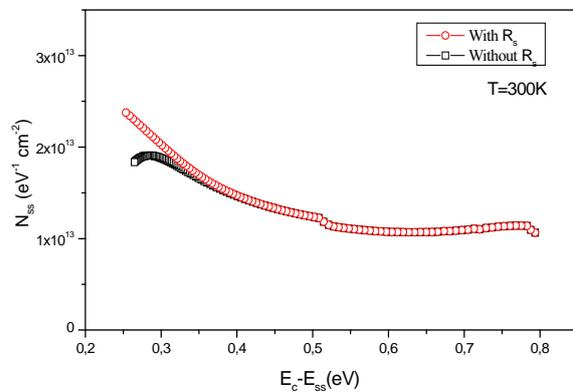
Fig. 7. The energy distribution profiles of  $N_{ss}$  as a function of  $E_c - E_{ss}$  extracted from the forward bias I-V data of the (Mo/Au)–AlGaIn/GaN HEMTs at room temperature.
