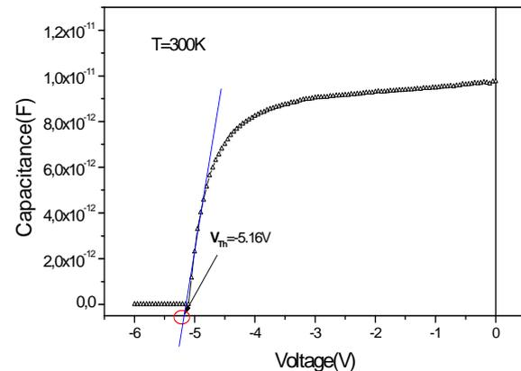
**Fig. 4.** The C-V characteristics (Mo/Au)-AlGaN/GaN HEMTs of the measured at T = 300 K.
