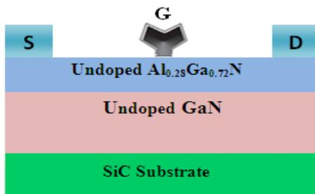
Fig. 1. Schematic of Al<sub>0.28</sub>Ga<sub>0.72</sub>N/GaN HEMTs.
