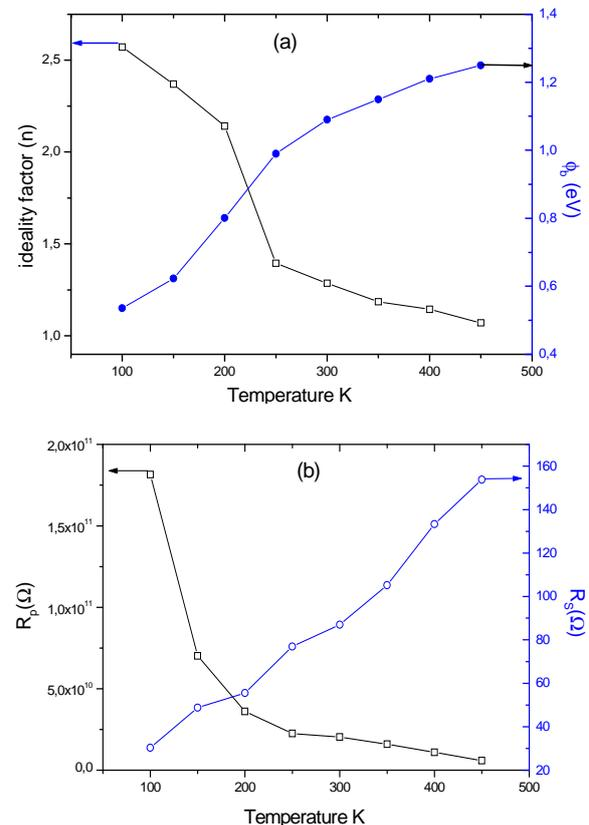
Fig. 3. (a) The values of  $\Phi_b$ ,  $n$  and (b) The values of  $R_s$ ,  $R_p$  at various temperatures of a (Mo/Au)-AlGaN/GaN HEMTs.
