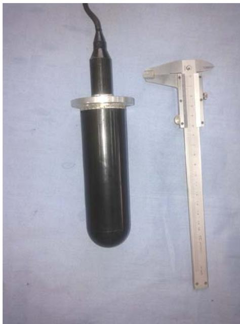
Fig. 6. The acoustic vector sensor.
