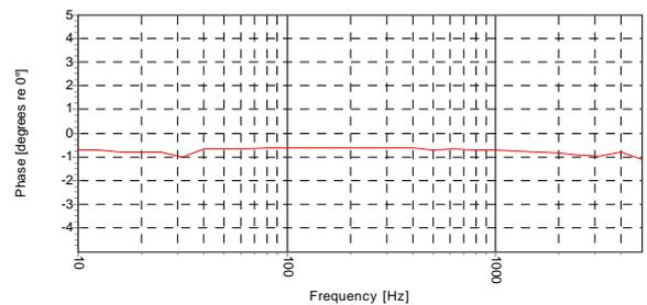
(b) Fluctuation curve of the accelerometer phase
