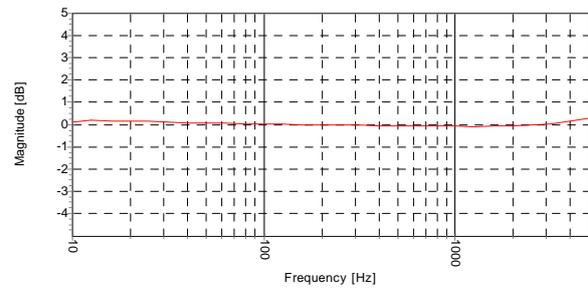
(a) Fluctuation curve of the accelerometer sensitivity
