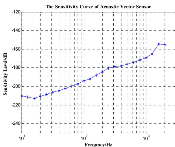
Fig. 7. The curve of the acoustic vector sensor sensitivity.
