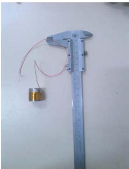
Fig. 3. The designed accelerometer.
