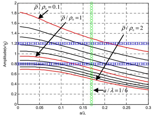
Fig. 1. The character curve of velocity ratio of the cylindrical vector sensor.
