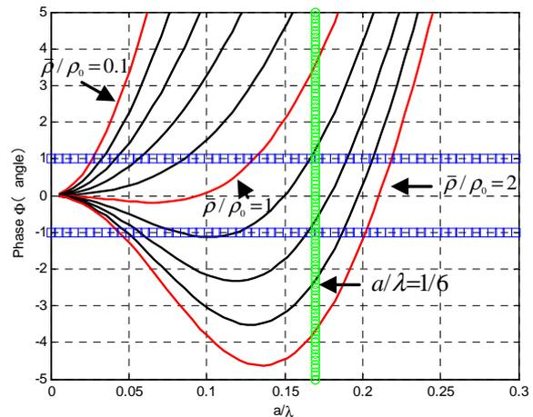
Fig. 2. The character curve of phase of the cylindrical vector sensor.
