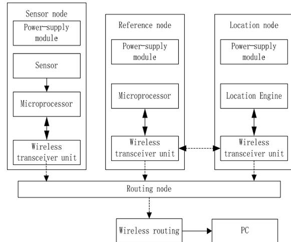
Fig. 2. System hardware structure diagram.
