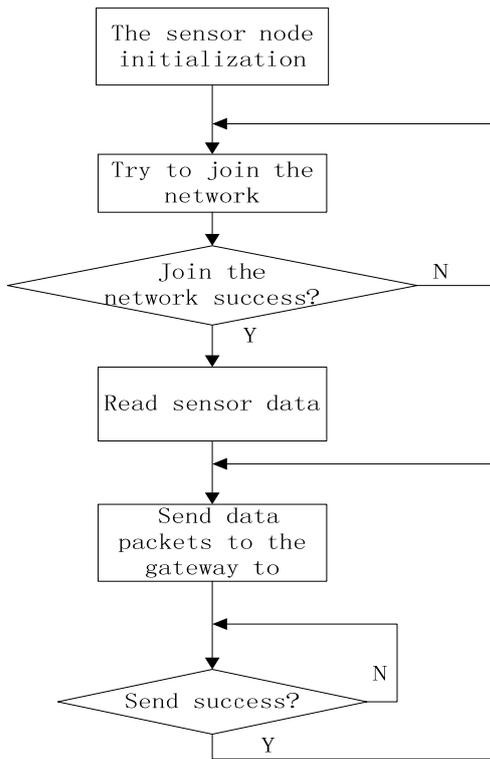
Fig. 3. Sensor nodes workflow.
