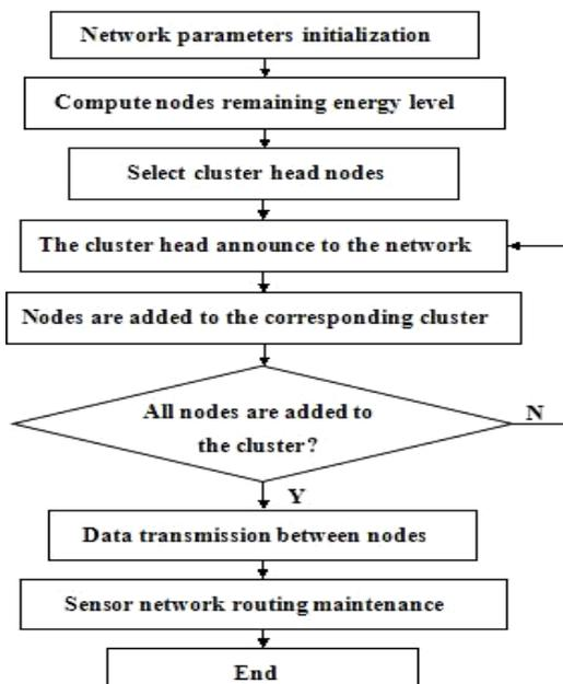
Fig. 1. The improved LEACH routing algorithm workflow.
