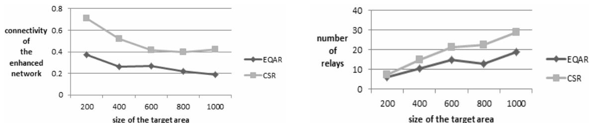
Fig. 4. Connectivity and relay number of EQAR and CSR against size of the target area (3 segments).
