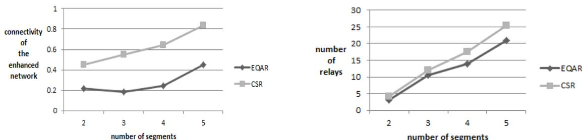
Fig. 3. Connectivity and relay number of EQAR and CSR against number of segments (size 300).
