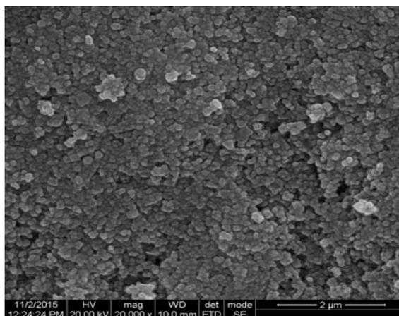
**Fig. 2.** SEM images of ZnO nanoparticles.
