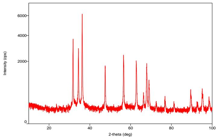
**Fig. 1.** XRD spectra of ZnO nanoparticles.
