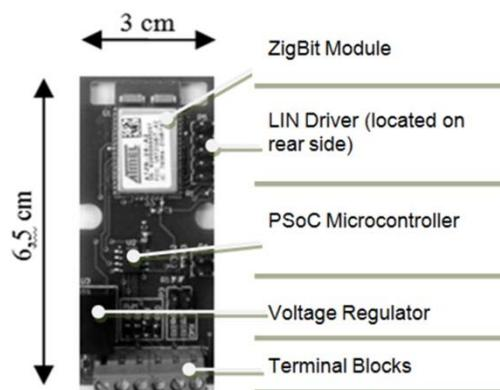
Fig. 12. The front side of the LEDWIRE Master node with ZigBee gateway capability.
