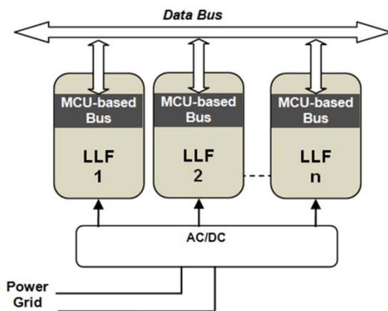
**Fig. 7.** RGB color control topology for a cluster of LLFs based on the bus topology.
