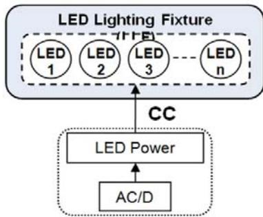
**Fig. 2.** LED lighting fixture (LLF) powered from an external constant current power supply unit.
