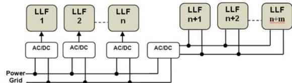
**Fig. 4.** Constant voltage power supply in dedicated and string power distribution topologies.
