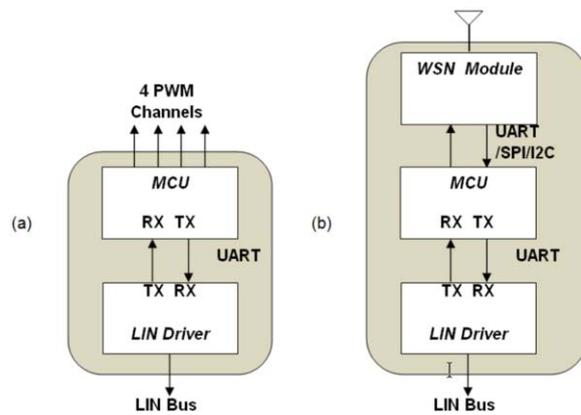
Fig. 10. (a) The LEDWIRE Slave node, (b) the LEDWIRE Master node.
