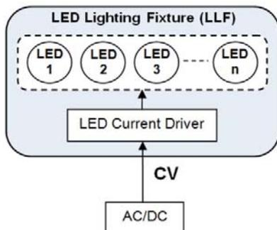
**Fig. 3.** LED lighting fixture (LLF) with LED power driver onboard (LDoB architecture) and external constant voltage power supply unit.
