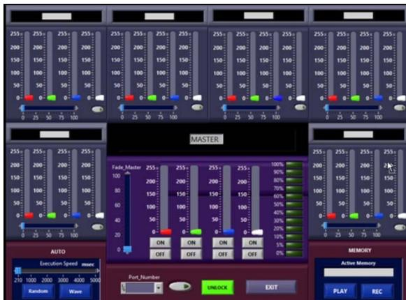
**Fig. 13.** The LabVIEW-based software GUI for LEDWIRE network platform testing.
