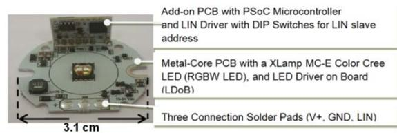
Fig. 11. The LEDWIRE Slave implementation onto a LED engine.
