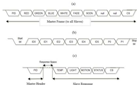
**Fig. 9.** The Global Command (a), the Protected Identifier (PID) field (b), and the Status Command followed by a Slave's response (c).
