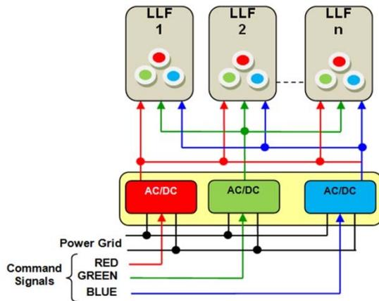
**Fig. 6.** RGB LED lighting fixtures (LLFs) clustered according to the drive of each particular color.
