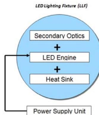
Fig. 1. The main parts of a LLF.
