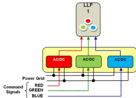
**Fig. 5.** The power supply topology for a RGB LLF.
