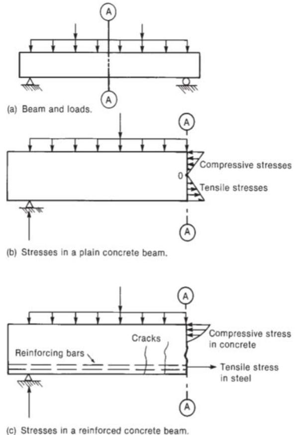
Fig. 2. Plain and reinforced concrete beams [7].
