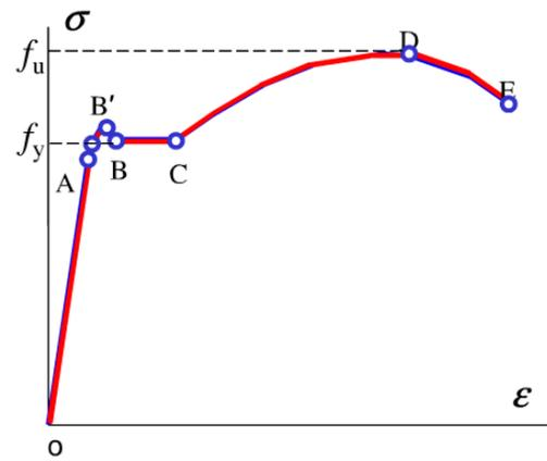
Fig. 4. The strain-stress curve of rebars.
