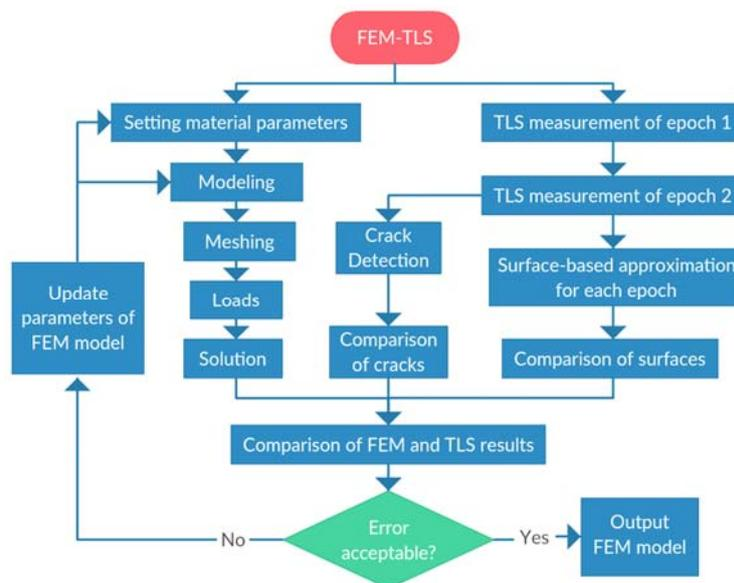
Fig. 1. The processes of FEM calibration based on TLS measurement.
