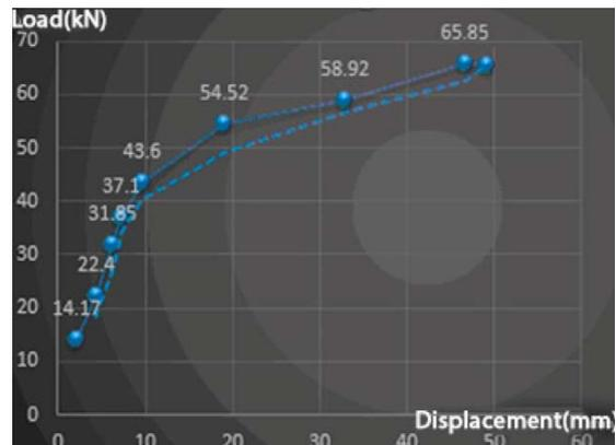
Fig 5. The load-displacement curve [10].
