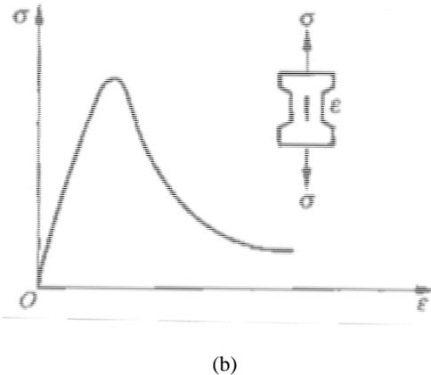
Fig. 3. The stress-strain curve of concrete in uniaxial compression and tension [8].
