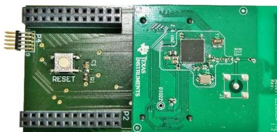
**Fig. 5.** CC2650 EM Board and Stack Adapter.
