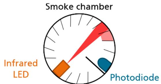
**Fig. 3.** Schematic of a photoelectric smoke detector.
