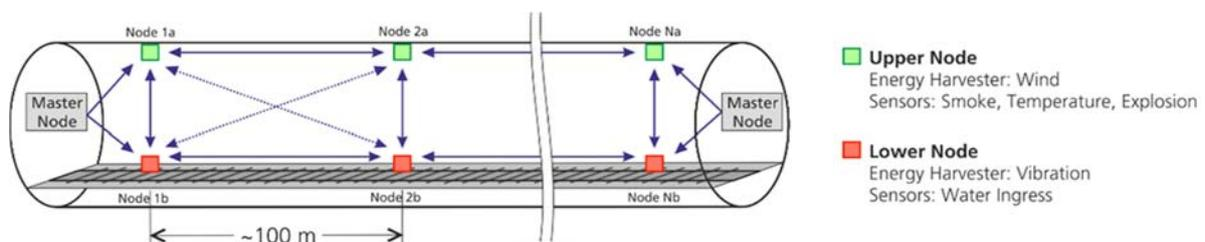
Fig. 1. Applied WSN topology in underground tunnel.
