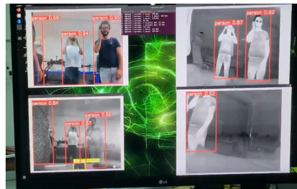
Fig. 12. Output of the YOLOv5 Algorithm with NVidia Jetson Xavier Nx.
