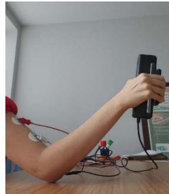
Fig. 4. Display of the 80^\circ position of the elbow angle during measurement.
