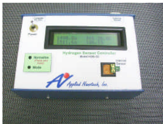
Fig.8. Picture of ANI's sensor mounted on the controller.
