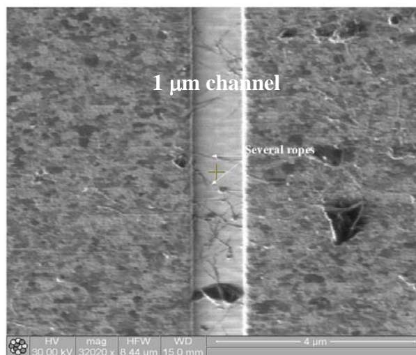
Fig. 3. A channel, 1 μm width, has been milled by FIB transversally to a Cr/Au pad, previously evaporated by e-beam. SWCNT ropes/DMF suspension has been deposited on channel.
