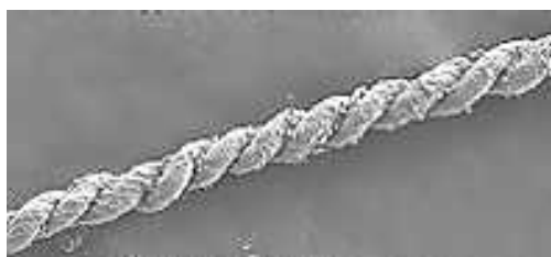
Fig.1. SEM image of a single SWCNTs rope [11].
