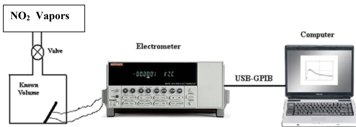
Fig. 2. Experimental setup for sensing \text{NO}_2 vapors at room temperature using Keithley Electrometer interfaced with computer.
