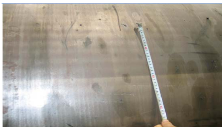
Fig. 1. The shape of chatter marks on backup rolls surface.
