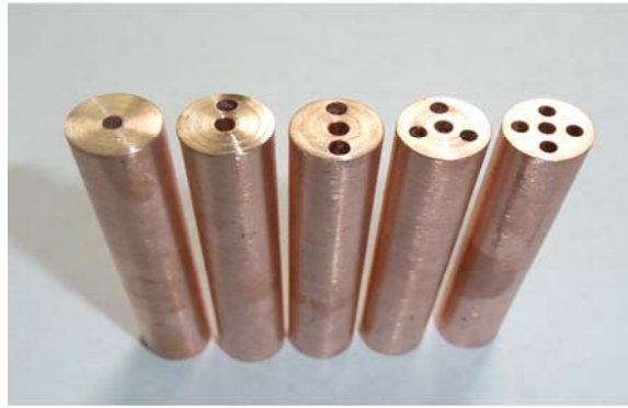
Fig. 3. Photograph of the multihole cylindrical electrode with different number of holes.
