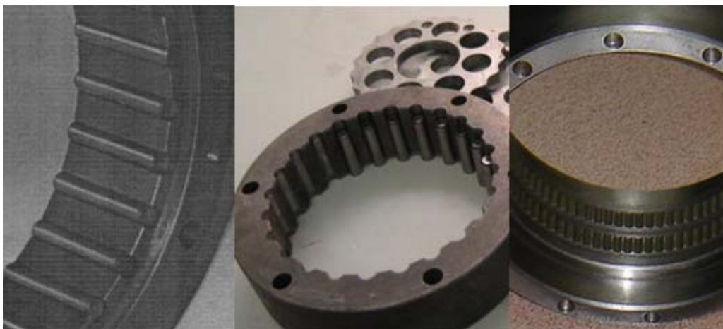
Fig. 4. The teeth of the pin gear designed as cylinders in half-embedded.
