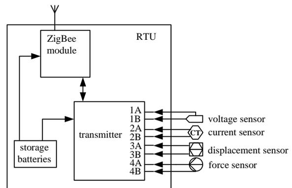
Fig. 4. The structure of the slave station.
