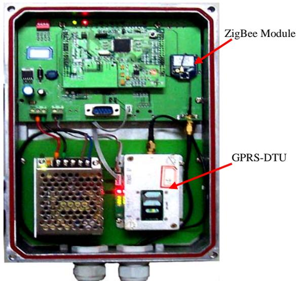
Fig. 5. The hardware of the master station.
