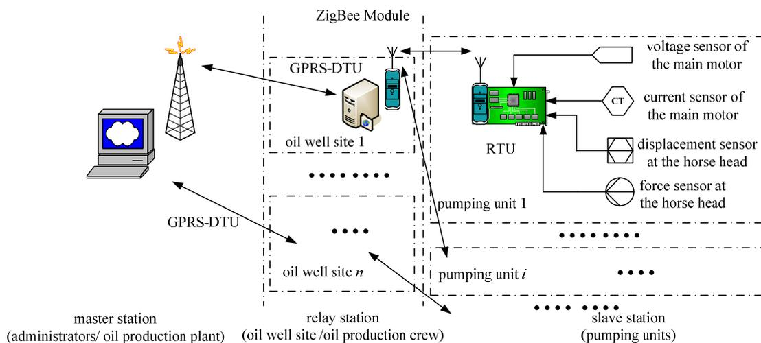
Fig. 3. The structure of the sensing network.
