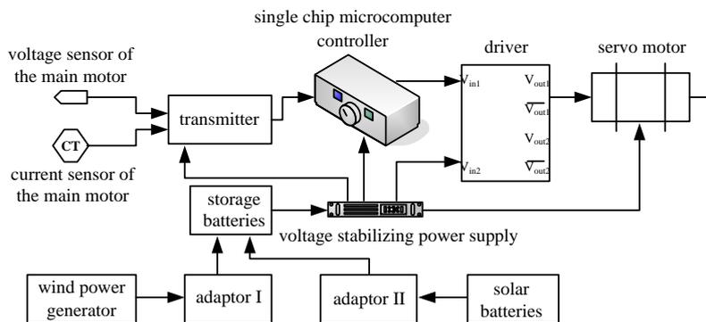
Fig. 2. The structure of the control system.
