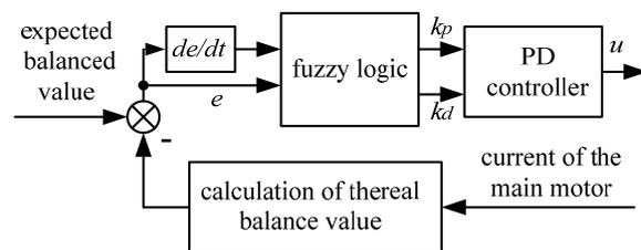
Fig. 6. The structure of signal processing for the current sensor of the main motor.
