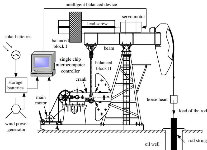
Fig. 1. The whole structure of the intelligent balanced device.
