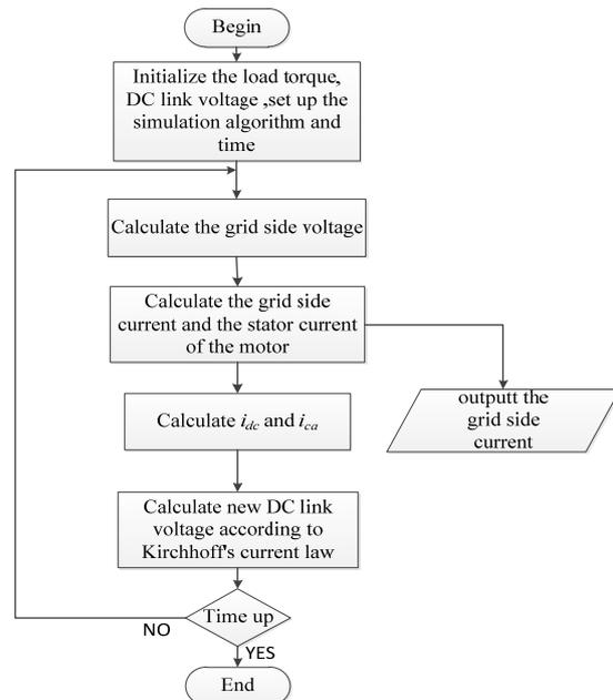
Fig. 2. The calculation flow chart.
