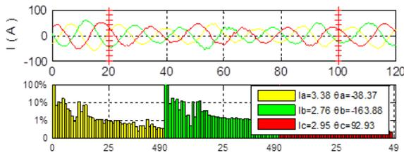
(a) the grid side current and its spectrum when the motor works at 15 Hz.
