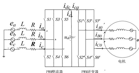
Fig. 1. Schematic of double PWM speed control system.
