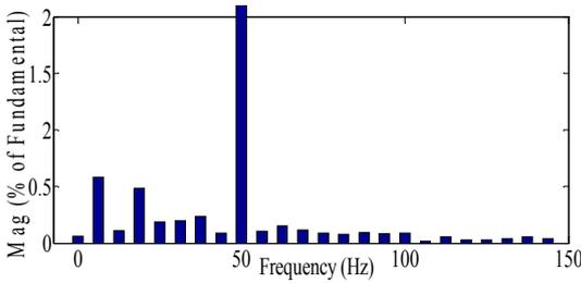
(b) the spectrum of grid side current when the motor works at 45 Hz.
