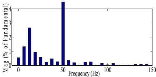
(a) the spectrum of grid side current when the motor works at 15 Hz.
