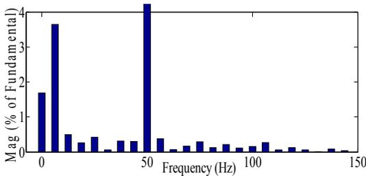
(b) the spectrum of grid side current when the motor works at 45 Hz.
