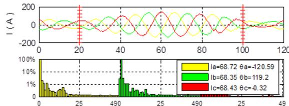
(b) the grid side current and its spectrum when the motor works at 45 Hz.
