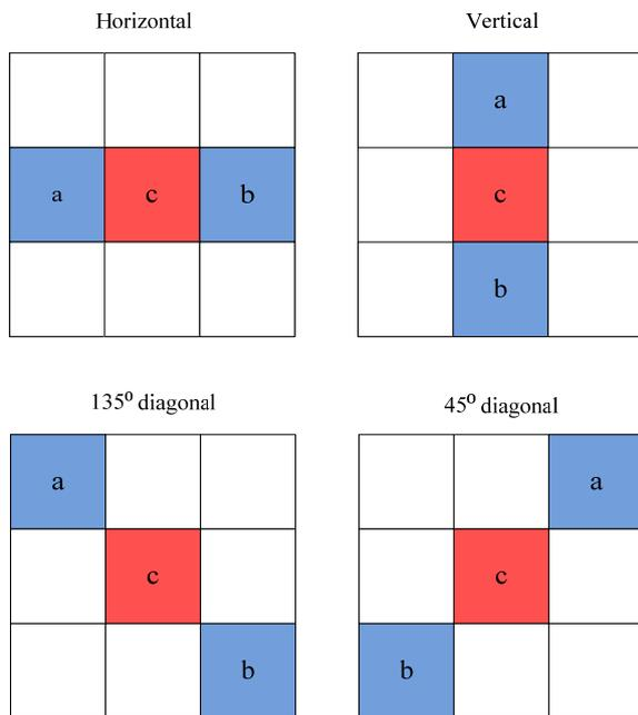
**Fig. 1.** Four 1-D directional patterns for EO sample classification: horizontal (EO class=0), vertical (EO class=1), 135° diagonal (EO class=2), and 45° diagonal (EO class=3).
