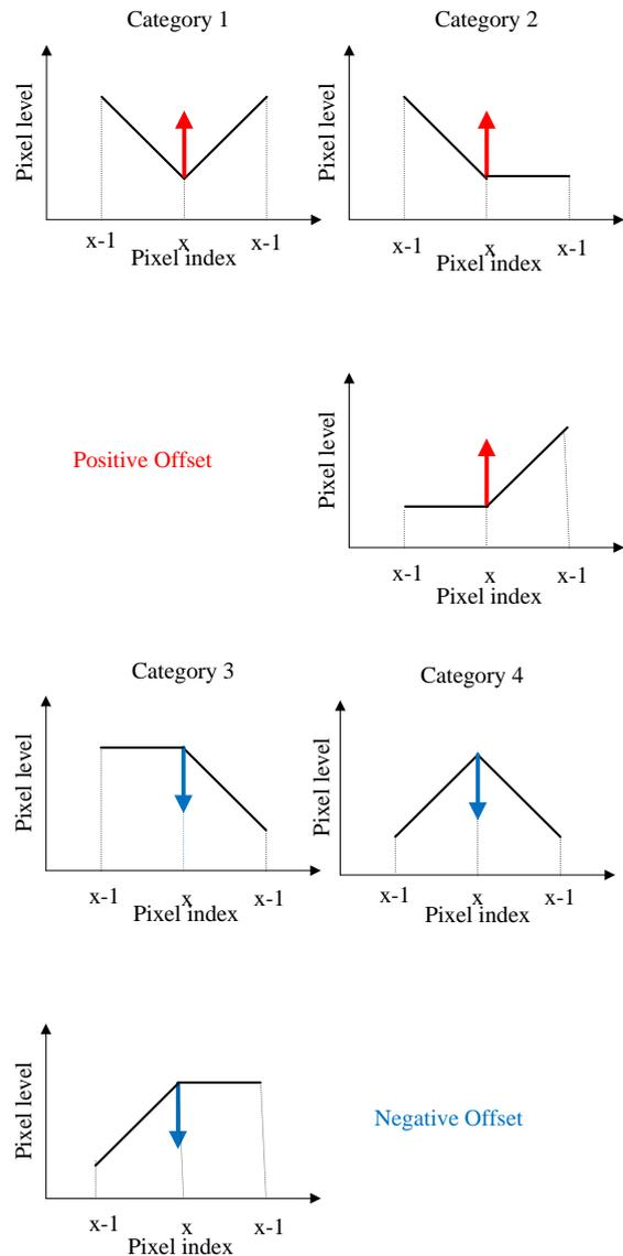
**Fig. 2.** Positive offsets for EO categories 1 and 2 and negative offsets for EO categories 3 and 4 result in smoothing.
