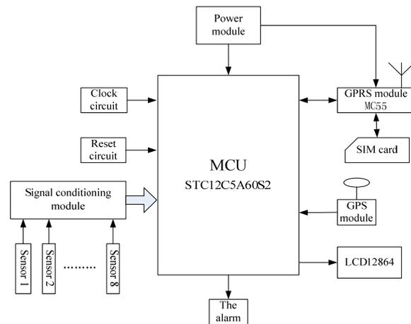
Fig. 2. The structure diagram of the remote terminal system.
