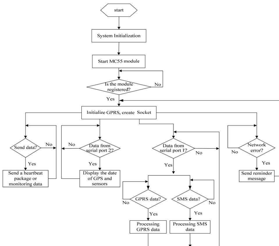
Fig. 6. The main program flow diagram.
