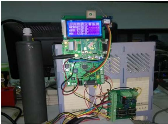
Fig. 7. The experimental platform connected with sample machine.
