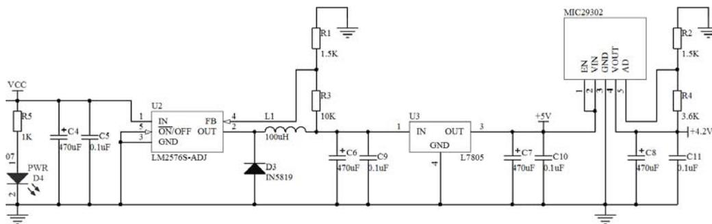
Fig. 5. The circuit diagram of the power module.
