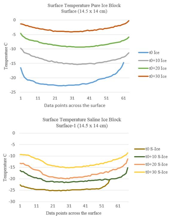
Fig. 6. Surface temperature profiles of Pure and Saline Ice block simultaneously observed from IR image under similar conditions.
