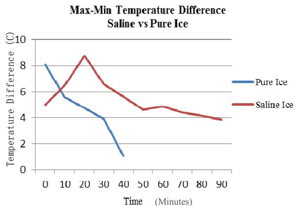
Fig. 10. Absolute maximum and minimum temperature difference (Saline vs Pure Ice).
