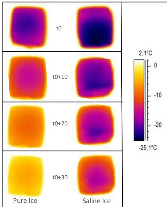
**Fig. 7.** Images of pure and saline ice blocks from thermal IR signature recorded under similar conditions.
