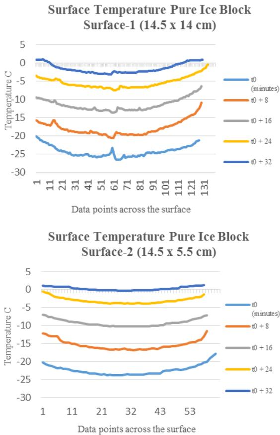
Fig. 4. Surface temperature of Ice block recorded from thermal IR signature at different intervals.
