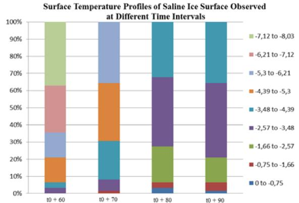
Fig. 9. Surface temperature profiles of saline ice block for rest of the time period (t0+60 onwards).
