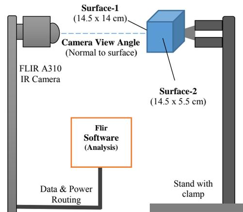
Fig. 3. Lab setup of pure ice block thermal signature evaluation.
