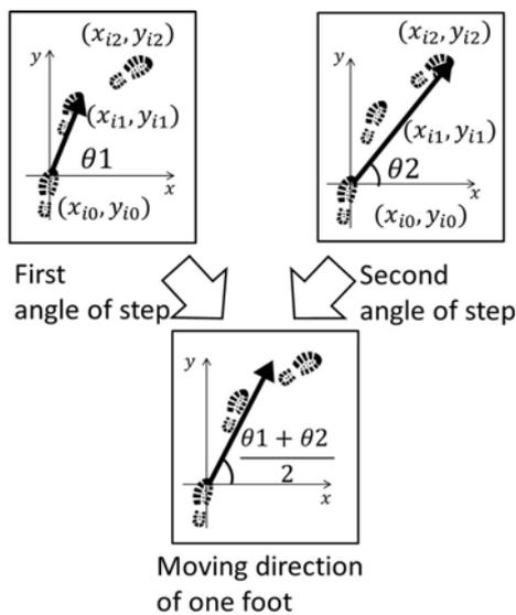
Fig. 3. How to derive the angle of the step.
