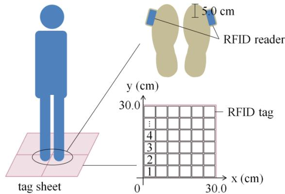
Fig. 3. Localization system using RFID.
