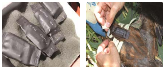
Fig. 11. Photo of devices ready to be used; “encapsulated” using two layers of thermo-contractile sleeve in opposite directions and in between a layer of silicone (left). Test with cranes; placement of a tracking device (right).
