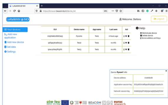
Fig. 4. Admin Webpage of the LoRaWAN portal. The Web portal consists of a Java Web Application running on Apache Tomcat.
