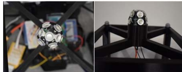
Fig. 1. 'Omnidirectional' US transducer array for the emitter.
