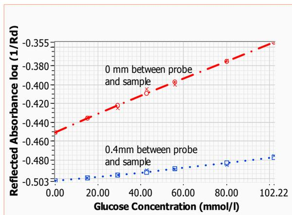
**Fig. 8.** Changes of the diffuse reflected absorbance with fresh milk + D-MEM (1x) liquid at different probe-to-sample distances.
