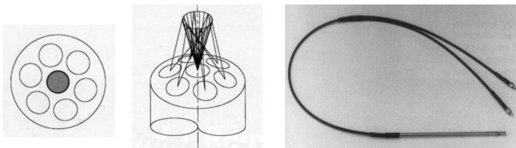
**Fig. 2.** End face of the optical fibre probe.
