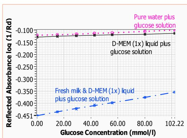
Fig. 7. Relationships between the diffuse reflected absorbance  $\log(1/R_d)$  and glucose concentration.
