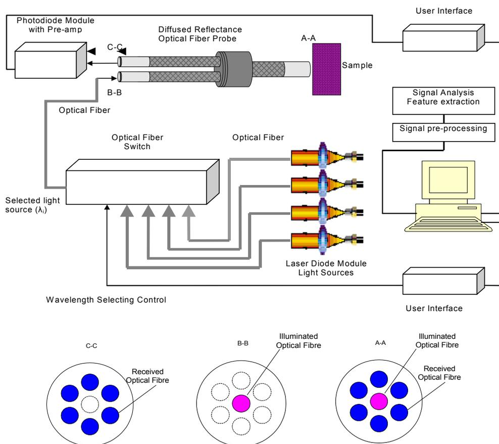
**Fig. 1.** Experimental layout.
