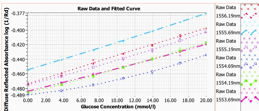
**Fig. 10.** Relationships between the diffuse reflected absorbance  $\log(1/R_d)$  and the glucose concentrations at different wavelengths with water mixed milk.
