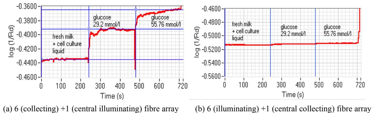
**Fig. 5.** Experiments of different fibre layout with fresh milk plus cell culture liquid medium.
