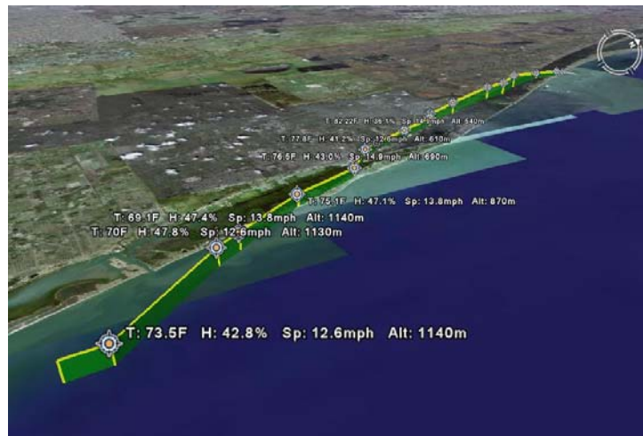
Fig. 6. Google Earth™ visual summary of free flight test on 19 April 2007. Data values were entered into the Google Earth™ image including temperature (T), humidity (H), speed (Sp), and altitude (Alt).
