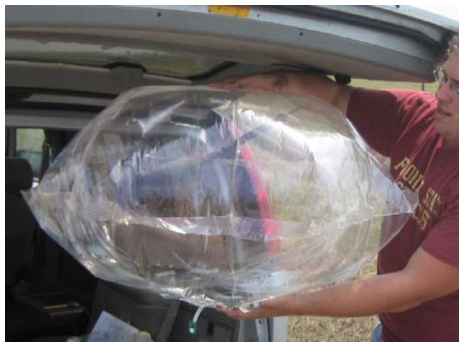
Fig. 1. The GEMS probe prior to deployment for the first successful free flight test. Note the electronics mounted on the bottom of the probe with the sensor board hanging below the balloon.
